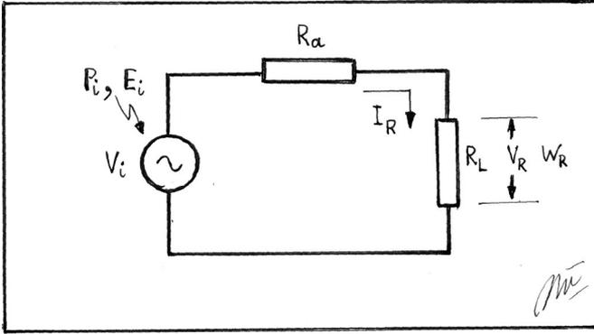
Fig. 2. Receiving antenna equivalent Thevenin circuit.
