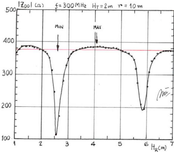
Fig. 9. Free space intrinsic impedance as a function of receiving antenna height  $H_R$ .
