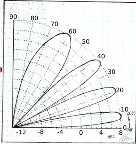
Fig. 6. Half-wave dipole transmitting antenna radiation pattern gain as a function of elevation angle at  $f = 300$  MHz.
