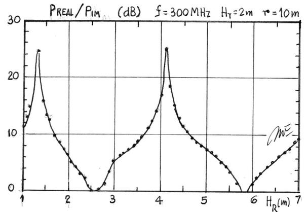
Fig. 8. Radio link power density relationship as a function of receiving antenna height  $H_R$ .
