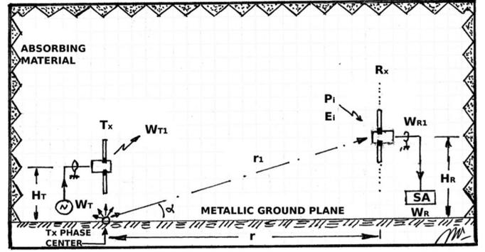
Fig. 11. Half-wave dipole antenna measurements setup (INTI Buenos Aires, Argentina).
