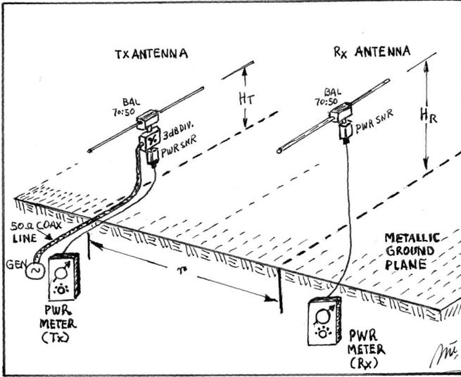
Fig. 4. Power measurement set up.
