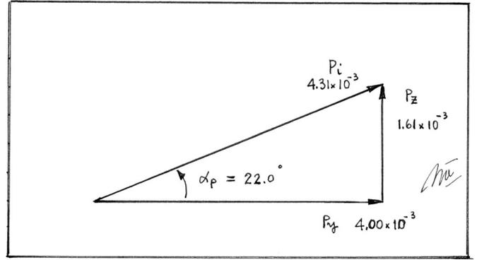
Fig. 7. Radio link power density components at a receiving antenna height  $H_R = 4.1$  m and  $f = 300$  MHz.
