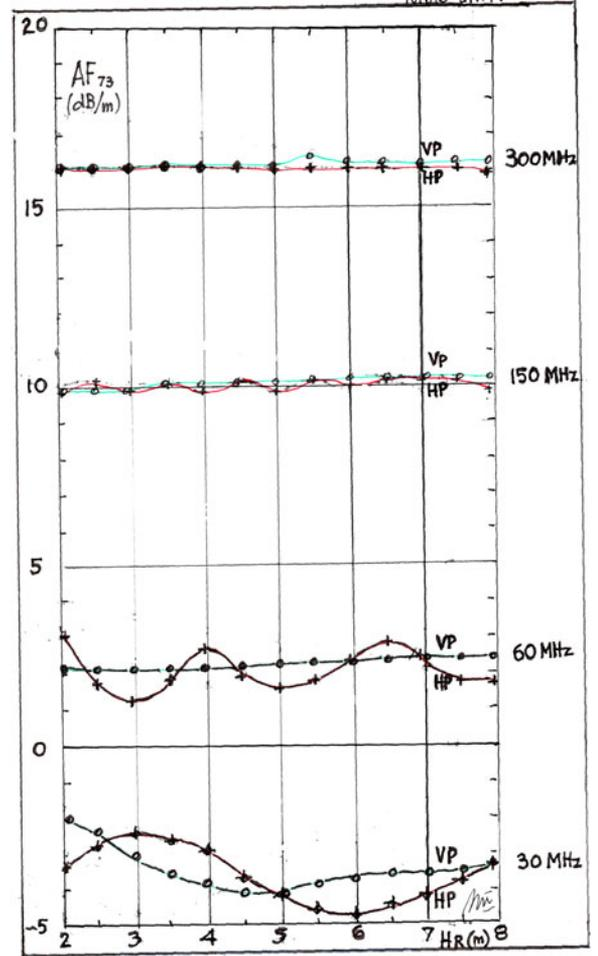
Fig. 3. Receiving antenna factor at  $r = 30$  m for horizontal and vertical polarization as a function of the receiving antenna height  $H_R$ .
