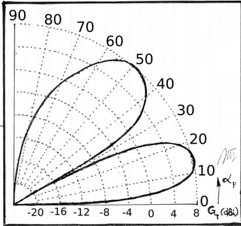
Fig. 13. Half-wave dipole transmitting antenna gain calculated as a function of elevation angle  $\alpha$  at  $f = 150$  MHz.
