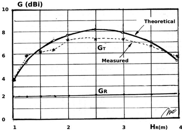
Fig. 12. Calculated and measured gain of two half-wave dipole antennas in a semi-anechoic chamber.
