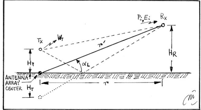
Fig. 1. Radiolink geometry.
