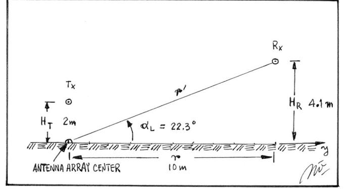
Fig. 5. Radio link elevation angle at maximum received power  $W_R$ .
