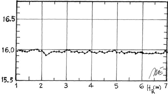
Fig. 10. Calculated receiving antenna factor  $AF_{R73}$  as a function of receiving antenna height  $H_R$  (dB/m) at  $f = 300$  MHz.
