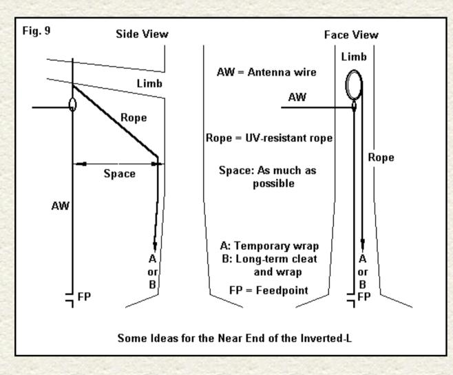
As shown in **Fig. 9**, we need to devise an installation that places the vertical section of wire as far from the tree trunk as may be feasible. We can use the same general support system, but notice that the wire does not run over the tree limb. Rather, it runs through a ring supported by the rope that we attach to the tree and pass over a handy limb. If you have two trees, then suspending a rope between them and running the
