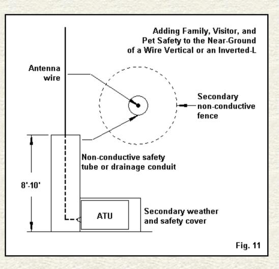
At the feedpoint end of the system, the tuner has an additional protective housing connected to the conduit. The housing serves several purposes. First, it prevents contact with the antenna terminals. Second, it allows us to elevate the tuner above ground to prevent the unit from
